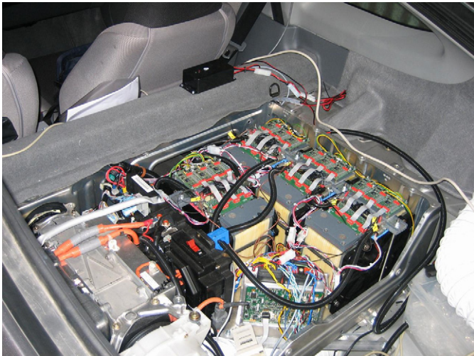
Fig. 4. Effpower bipolar lead-acid battery installed within the space vacated by the NiMH battery taken from Honda Insight No 2.
